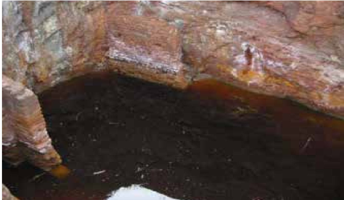
Acid mine drainage due to oxidation of pyrite at a copper mine
