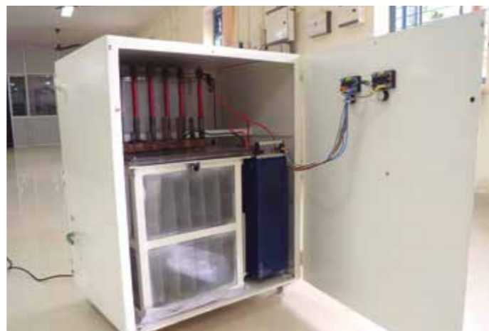
Photo 1 : Continuous electrochemical flow reactor (India)
